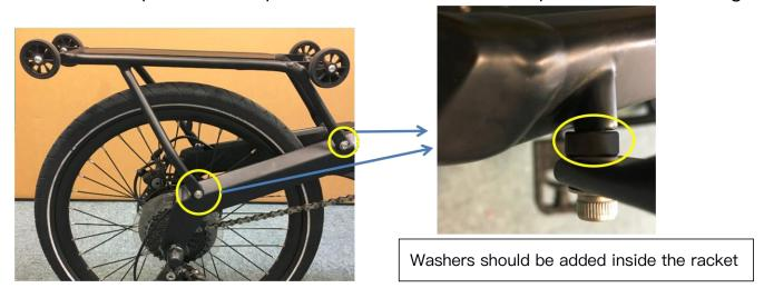
2.12.3 Lock the four screws with 5Nm of torque force to complete the assembly of carrier.
