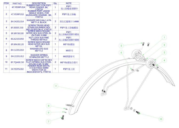
2.11.1 Install the front and rear wheels onto the fender (mind the directions of installing, as is shown in the following). The orders of spare parts are shown in the exploded-view drawing. The torsion force of locking is 3Nm.
