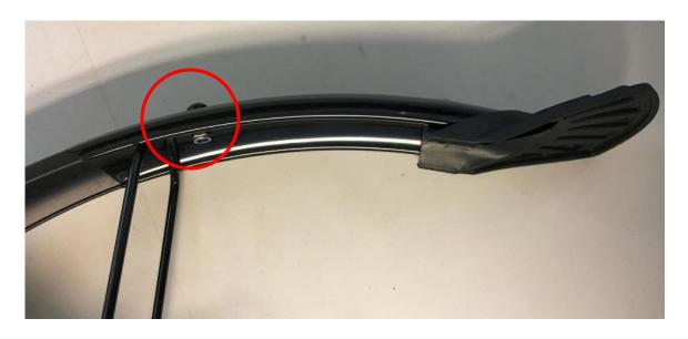
2.10.3 Install the hanger into the eyelet behind the front fork. The orders of spare parts are shown in the exploded-view drawing. The torsion force of locking is 3Nm (do not lock up the screw. Just insert it).
