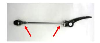
Note: the handle of quick release is on the right side of bike
