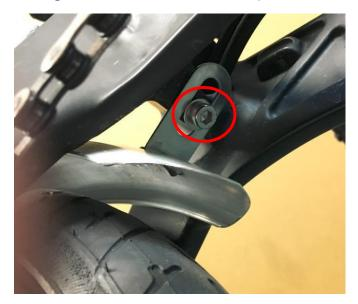
2.11.3 Install the fender onto the left and right attachment near the rear fork. The orders of spare parts are shown in the exploded-view drawing. The torsion force of locking is 5Nm (do not lock up the screw. Just insert it)
