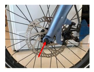
The disk needs to be stuck in the center of calliper.
