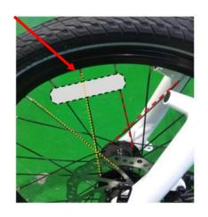
2.6.2 Use one left and two right spokes to jam the reflector and push it to the outside of the wheel as much as possible.
