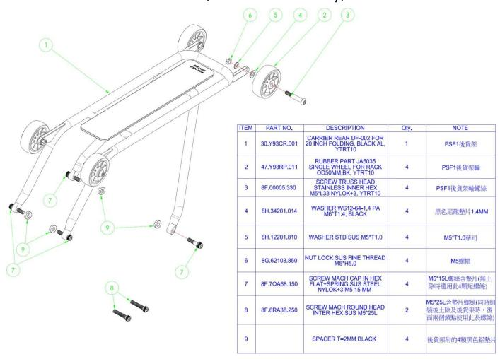
2.12.1 Remove the foldable bracket off (Properly keep the removed bracket. If the carrier is not installed, the bracket should be assembled for folding and standing).
