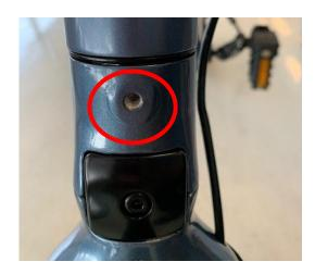
2.7.2 After headlamp is installed on the bracket, lock it into the keyhole of front fork with M6 screw/washer/spring washer in the accessory package.
