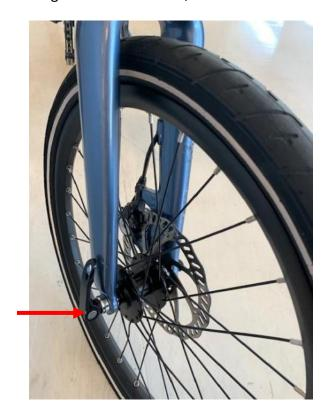
Press the handle of quick release upward and parallel it with front fork.
