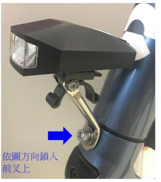
Insert the nut into the front fork according to the figure.
