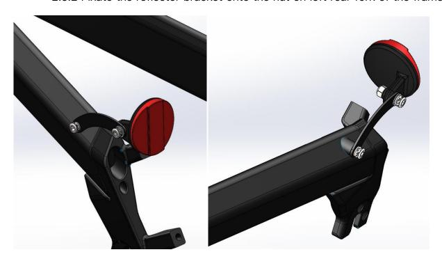
2.5.3 Place the reflector on the inside, and fixate the screw from the outside onto the inside with the nut.
