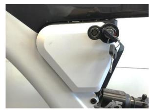
2.4.3 Press the key and turn it to "OFF". lock up the battery and assemble it.
