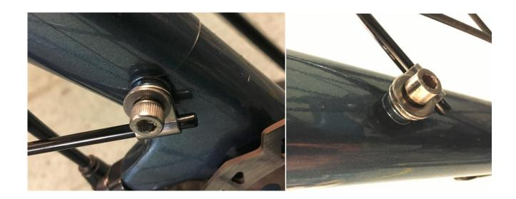
2.10.5 Adjust the fender properly, lock the screw up with torsion, wrap the protection pack on the front fork and complete the assembly of front fender.
