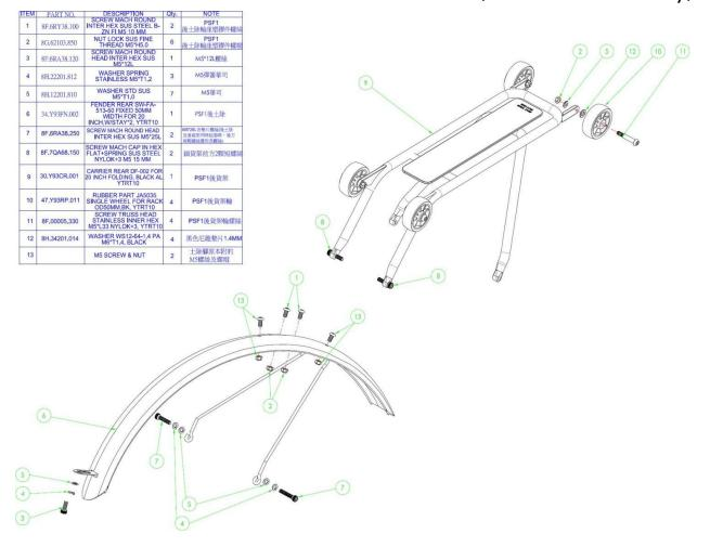
2.13.1 Install the rear fender (note the direction of installation in the following figure), original wheels, front fixed orifices, screws and nuts and orders of other spare parts are shown in the exploded-view drawing. The force of torque is 3Nm.
